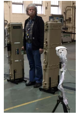
Figure 4-3 PPVM with camera set up in pedestrian mode
