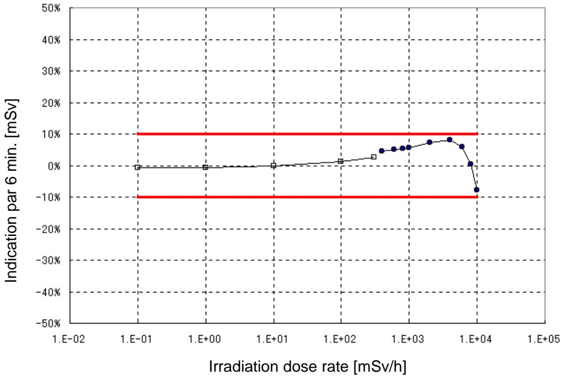
Open square is experimental data, black circle is simulated data using electric pulses.
