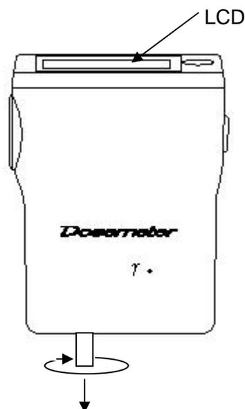
Please entry a new battery (CR123A) into the dosimeter for the first time use. (To see Sec. 5.1 battery replacement)
