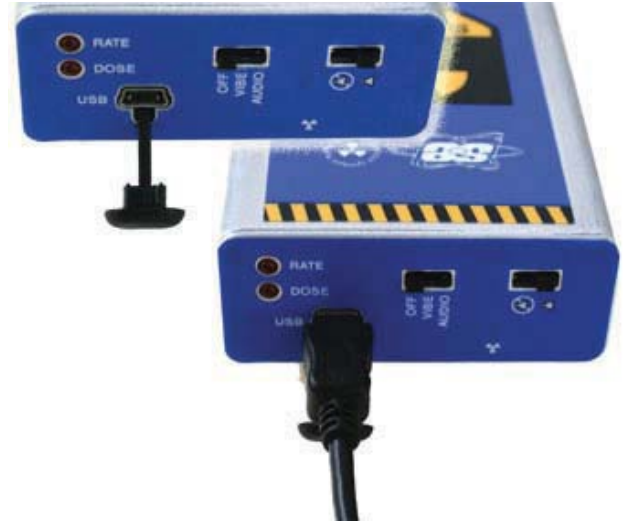
Fig 2. Unplug the mini-USB cap from the USB port and connect the mini-USB cable
